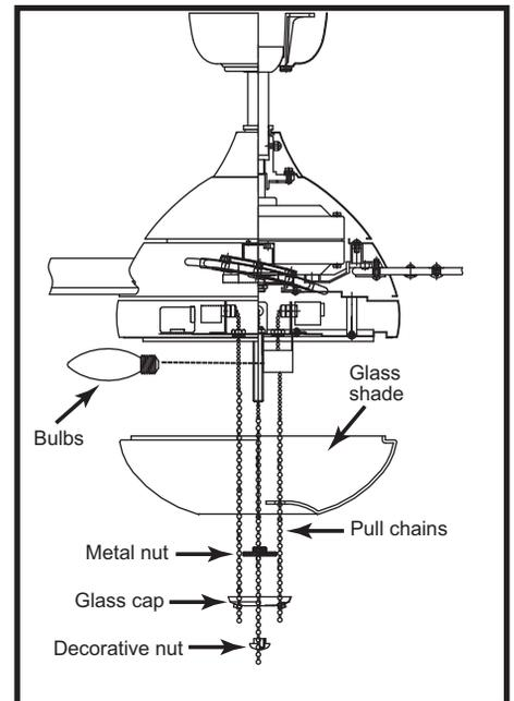
**4. Attaching the Light Kit (Fig. 12)** Connect the cannon plug from the motor assembly to the corresponding plug in the light kit. Attach the light kit to the mounting plate by using the three (3) screws provided that are preinstalled on the mounting plate.
