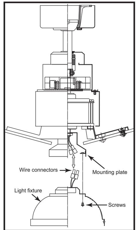
Attach the light kit to the mounting plate by using the three screws provided that are pre-installed on the mounting plate. (Fig. 11)
