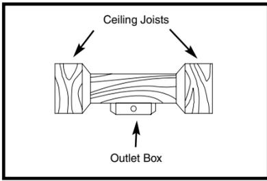
4. Figures 1, 2 and 3 are examples of different ways to mount the outlet box in different situations. A longer downrod may be required in sloped ceiling situations to maintain proper blade clearance.
